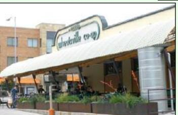
A cistern at the end of the patio collects rainwater from the awning gutter and two cisterns on the east side of the store collect rainwater off the roof. This not only allows us to water our landscaping, but also prevents hundred of gallons of runoff from running into storm sewers and our neighbors yards
